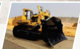
BD475-2 Bulldozer (FHP 642 kW)
