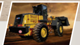
BL30-1 Front End Loader (Bucket 3.1 cum)
