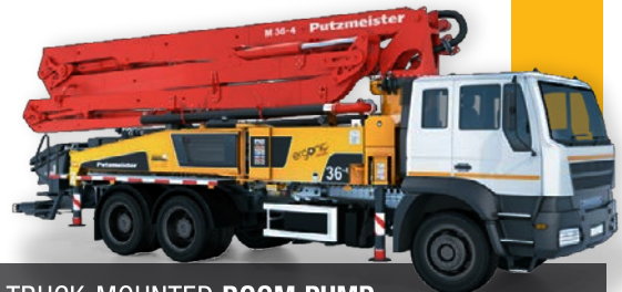
TRUCK-MOUNTED BOOM PUMP Vertical reach: 36 m | 42 m
