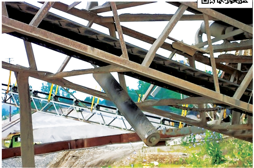
Unguarded return rollers over walkways can fall and produce a serious hazard.
