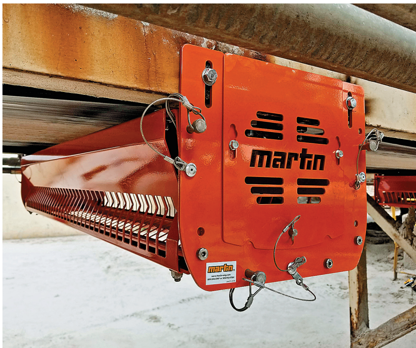
Return roller guards ensure detached rollers don't pose a hazard to workers or harm the system.
