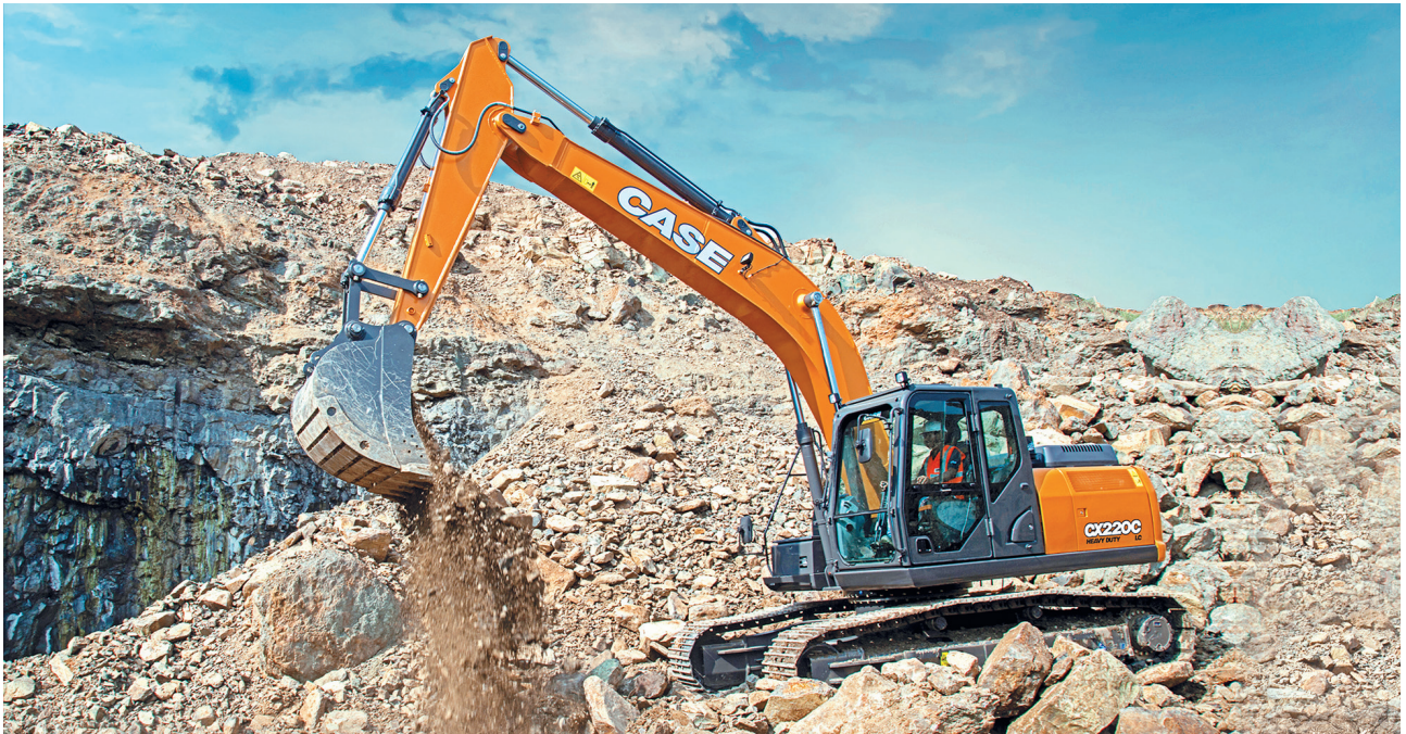
Compact excavators are similar to regular excavators in structure, with a crawler undercarriage and revolving superstructure fitted with a boom.
