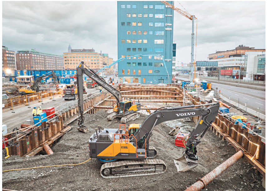
Volvo CE's large 30-tonne grid-connected electric excavator formed part of the Electric Worksite tests.
