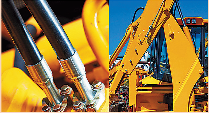
Manufacturers have moved to a reinforcement wire with an oval cross-section as opposed to a round, offering additional outside diameter and hose weight savings.
