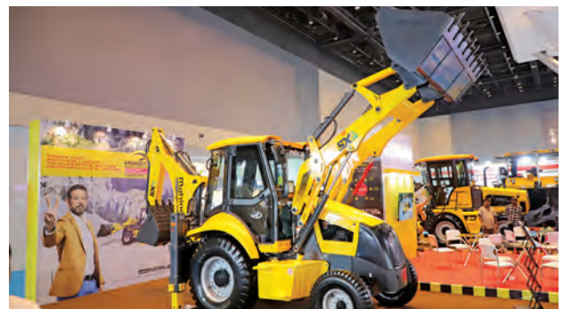
Mahindra EarthMaster backhoe loader SX Smart 50 comes with a 36.2 kW (50 HP), best-in-class fuel efficiency, and optimal backhoe performance.
