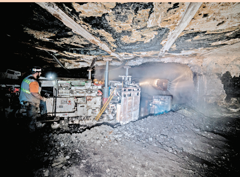
Worker using continuous miner to extract coal underground.
